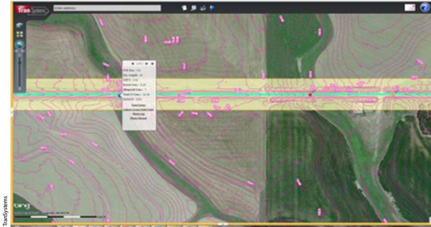
**Figure 2.** This LiDAR map shows a road segment in Barton County with 1 ft contours. The layers, developed by TranSystems, include the ROW shown in yellow and culverts shown as red dots on the road. Data attached to the culverts include size, characteristics, scour form, and a photo log. A cost-benefit analysis is under development to help prioritize projects.
