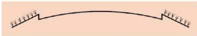
Fig 2. A parabolic crown caused by worn blades. The outer edge of the road slopes too much and the center is too flat. Gouging causes high shoulders.
