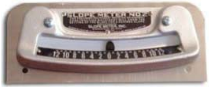
Figure 3. A slope meter accurately displays the percent of cross slope.
