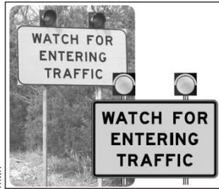
In Missouri these signs have cut stop-controlled intersection crash rates in half and have reduced severe crashes by 77 percent at those locations. The technology is also used in North Carolina where it has been reliable and easy to maintain. Similar devices have been installed at a few locations in Kansas. See sidebar at right.
